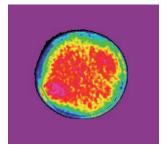
Beam profile in near field @ 355 nm, stable resonator
