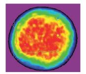
Beam profile in near field @ 1064 nm, stable resonator
