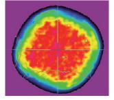
Beam profile in near field @ 532 nm, stable resonator
