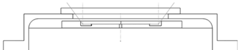
Figure 7: ‘Direct mount’ front end of Marana 4.2B-11, yielding f/# 0.7 and 72° Cone Angle. Discuss custom mounting flanges with Andor’s CSR Service.
