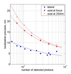
**Figure 3.** Localization precision dependence on the number of detected photons. Blue, lateral localization precision with optimized PSF and induced astigmatism; red filled circles, axial localization precision close to the focus; red empty circles, axial localization precision at + or - 250 nm away from the focus. The amplitude of astigmatism is 60 nm RMS. Solid lines are the fit of the data with a power law.
