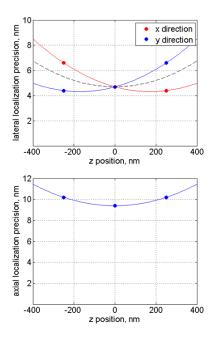
**Figure 6.** Dependence of the localization precision on the distance from the focal plane for the lateral (upper panel) and for the axial (lower panel) directions @4000 photons. The dashed line in the upper panel is the average of localization precisions in x and y directions.
