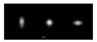
**Figure 4.** Image (averaged over 40 individual beads) of the PSF with 60 nm RMS astigmatism at -250 nm of the focus (left image), at the focus (center image), and at +250 nm of the focus (right image).
