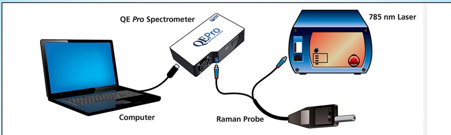
Figure 1: Modular fiber optic Raman spectroscopy system for SERS detection.
