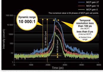
Single shot streak image with laser diode (Equipment used: C13410-01A/V12303-01/ORCA®-Flash4.0)
