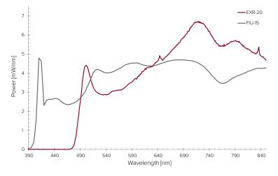
Visible power density curve of the high power lasers. Note: FIU-15's typical single mode fiber coupling efficiency is 70% above 450nm The SuperK EXTREME is available in four different variants:
