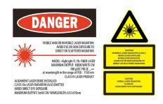
Coherent industrial lasers are designed in strict accordance with the respective safety regulations. We certify that each laser manufactured by our company complies with FDA Radiation Performance Standards, 21 CFR Subchapter J and with IEC 60825. Warning labels as shown in the figure appear on each Coherent laser to indicate the respective classification.
