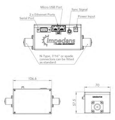
Figure 1: Dimensional drawings of the standard Octiv Mono (model 02-0231-01) with Quick Change RF connector interface. All dimensions are in mm. Contact Impedans for dimensional drawings of other models.
