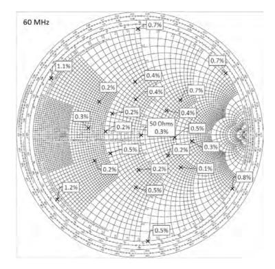
Figure 4: Typical 60 MHz impedance verification against VNA.
