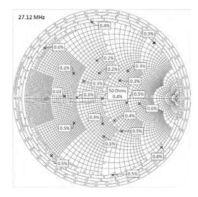
Figure 3: Typical 27.12 MHz impedance verification against VNA.
