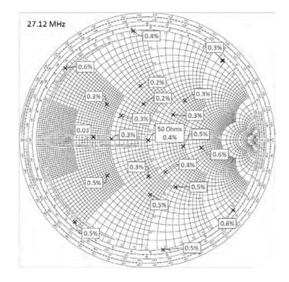
Figure 4: Typical 27.12 MHz impedance verification against VNA.
