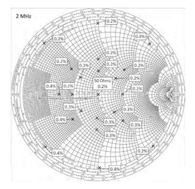
Figure 3: Typical 2 MHz impedance verification of an Octiv unit against VNA.
