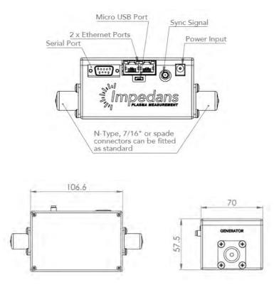
*Figure 1: Dimensional drawings of the standard Octiv Poly model 02-232-01 with Quick Change RF connector interface. All dimensions are in mm. Contact Impedans for dimensional drawings of other models.*
