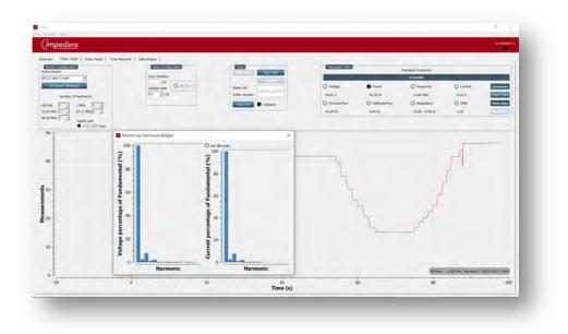
Figure 8: Example of the harmonic spectrum.
