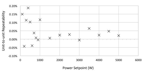
Unit-to-Unit Comparison, 5 kW Ramp, 13.56 MHz
