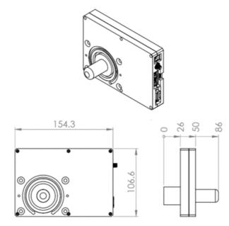
Figure 2: Dimensional drawings of model 02-0308-01.
