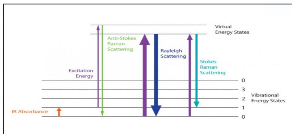
Raman scattering from a molecule results in light of a slightly longer or shorter wavelength than the excitation laser, with the energy difference corresponding to a vibrational energy level transition within the molecule.
