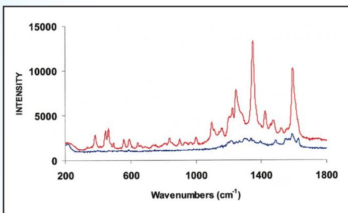
A 90:10 mixture of unmarked diesel-kerosene (blue trace) is easily distinguished from a mixture in which the kerosene diluting the diesel contains a marker (red trace).
