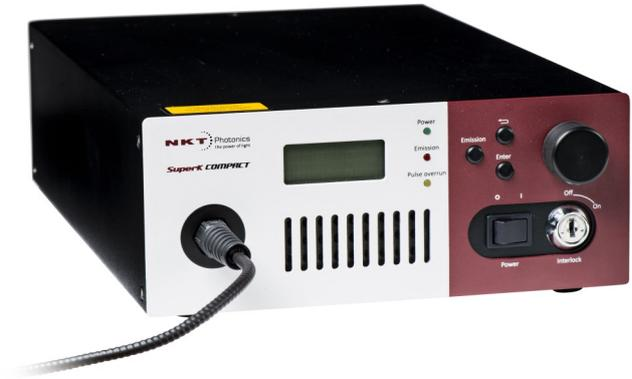
SuperK COMPACT is a cost efficient turn-key supercontinuum white light source with a wide output spectrum that covers the entire 450-2400 nm region. The output is single mode with a brightness many orders of magnitude larger than that of other white light sources like incandescent lamps and with far more bandwidth than ASE sources or SLEDs.
