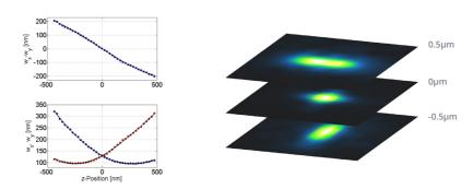
Left: A calibration curve obtained using MicAO 3DSR features aberration-free axial symmetry (lower panel) and high lateral separation of astigmatic PSF along the whole Z range (upper panel). Right: A representative stack of astigmatic PSF at three planes.
