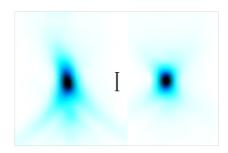
The axial view of a typical point spread function (PSF) before correction (left) and after correction (right) of aberrations. The correction of aberrations increases the axial symmetry of the PSF and almost doubles the amount of detected photons in the focus. This improves localization precision by 40% in all three dimensions. Scale bar is 300nm.
