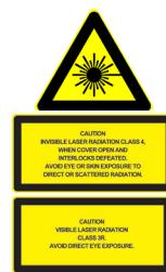
Coherent industrial lasers are designed in strict accordance with the respective safety regulations. We certify that each laser manufactured by our company complies with FDA Radiation Performance Standards, 21 CFR Subchapter J and with IEC 60825. Warning labels as shown in the figure appear on each Coherent laser to indicate the respective classification.
